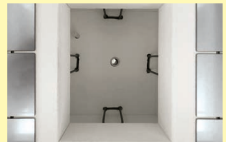
Furnace chamber heated on four sides for model LHT 01/17 LB Speed
