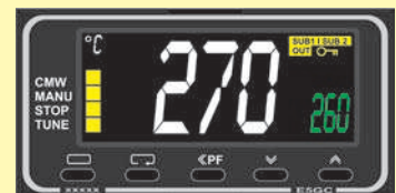
Example of an over-temperature limiter
