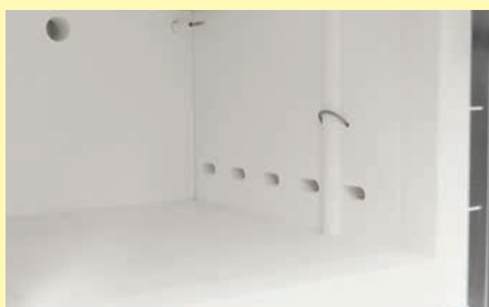
Furnace chamber with air inlet openings for air exchange of more than 6 times per minute
