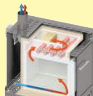
Schematic presentation of air circulation in ashing furnace L 24/11 BO
